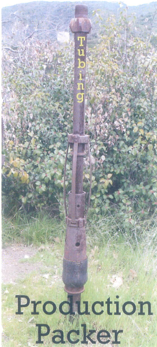
Hook Wall Pumping Packer (a type of production packer)
